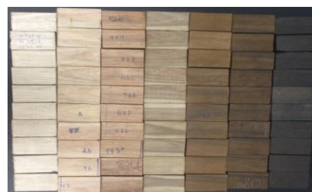
Figure 1 – Colour changes in wood caused by different thermal
